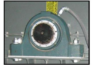
Bearing Sensor on Belt Conveyor
