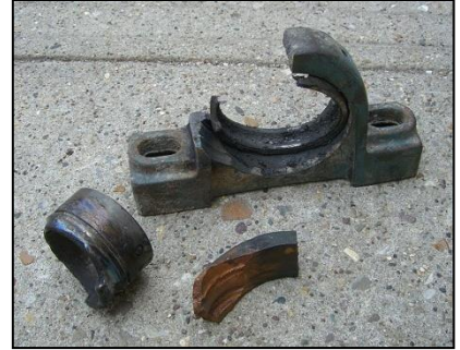
Example of Bearing Failure
