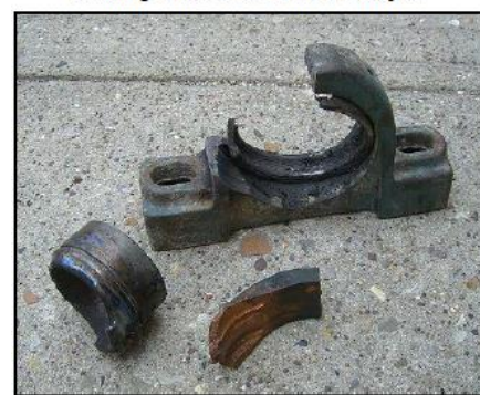
Example of Bearing Failure
