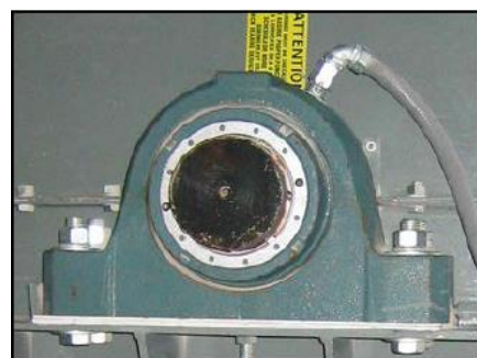
Bearing Sensor on Belt Conveyor
