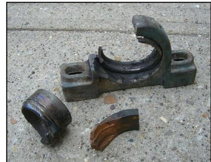
Example of Bearing Failure
