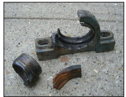
Example of Bearing Failure
