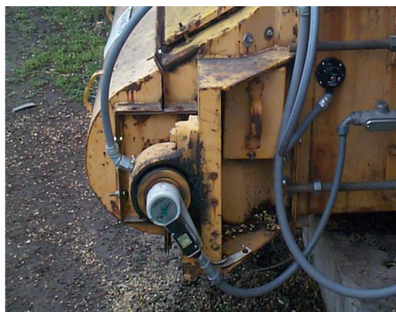
Whirligig installed on an enclosed belt conveyor shown with M800 speedswitch
